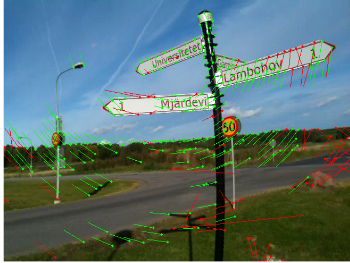
Figure 4.1: Tracked points between two frames. Rejected points in red, and accepted points in green.
