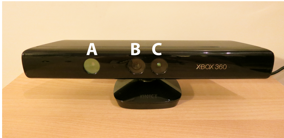
Figure 2.2: The Kinect Sensor, (A) NIR laser projector, (B) CMOS colour sensor, (C) CMOS NIR sensor
