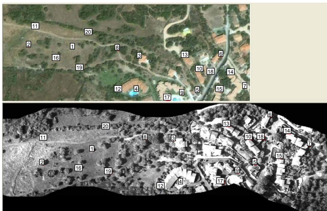
Figure 14. Map extracted from Google Earth employed for georeferencing both the mosaic and the images of the hyperspectral cube. The points employed for the geometric transformation are shown in white.
